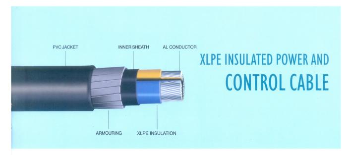
This is a thermoset type of polymer enriched with crosslinking agent. This is extruded over the conductor using modern extruders and is thoroughly crosslinked under controlled conditions. This XLPE insulation overcomes the drawbacks of PVC, hitherto extensively used as an insulating material, without losing any of PVC's desirable properties.
