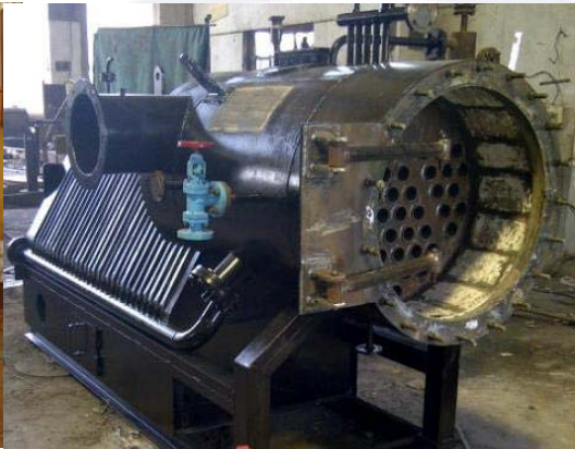
Membrane Wall SIB boiler
