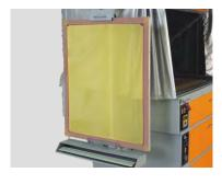
manually. This avoids any kind of shake while coating the emulsion on the screen ensuring trouble free operation plus saves one additional person for just holding the frame while other coats. This adjustable clamp locks
