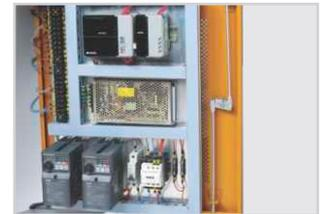
PLC (Programmable logic controller) and High Quality Electrical Components
