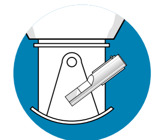
Scheme 3 Hydro-Probe II may be inclined down at approx 45° to minimise obstruction to the flow, when neck of bin is small.
