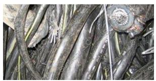
**Insulated Aluminum Wire**Aluminum Wire covered by jacket, free of steel.
