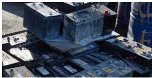
**Lead Batteries**No holes, battery intact. Labeled "PB" on fine print.
