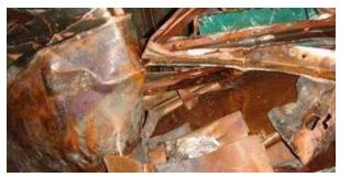
**Dirty Roofing Copper**Roofing copper with heavy tar, wood, or attachments.
