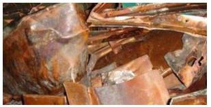
**#3 Copper with Tar**Roofing copper with heavy tar, wood, or attachments.
