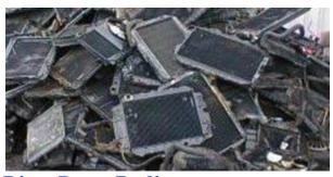
**Dirty Brass Radiators**Plastic or iron attached to radiators (no coolant).
