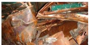
**Light Copper**Roofing/gutter/flashing copper with little tar or attachments.
