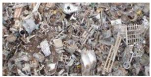
**Die Cast**Free of steel/iron/platic and melted pieces.
