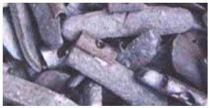
**Lead Wheel Weights**No iron clips attached.
