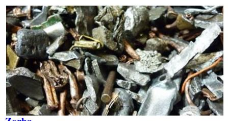
**Zorba**A heterogeneous mixture of aluminum and copper that remains after the shredded car has passed through the entire downstream operation.
