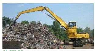
**#1 HMS**Prepared pieces smaller than 60"x 24" over 1/4" thick.
