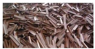
**#1 Steel**Prepared pieces smaller than 60"x 24" over 1/4" thick.
