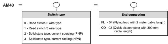
Ordering example :- AM40 - 0 - FL - 04 (2 wire Reed switch with Flying lead of 2 meter cable length)
