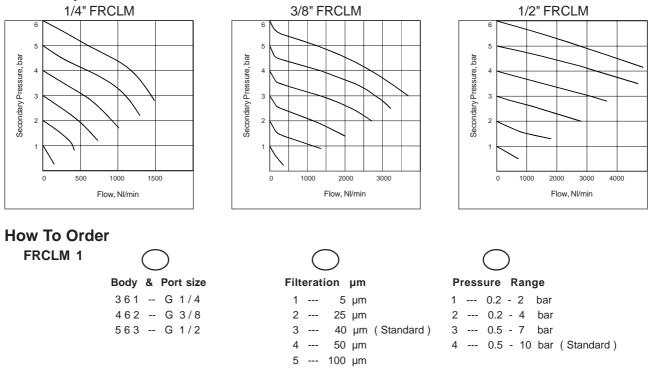
Ordering example : Filter Regulator Combination and Lubricator Modular - 3/8 size ( with G3/8 port ) with 5 µm Filter and pressure range 0.5 - 7 bar : Ordering No : FRCLM 146213. If ordered as 3/8 FRCLM, our standard model FRCLM 146234, with 40 µm Filter and pressure range 0.5 - 10 bar will be supplied.
