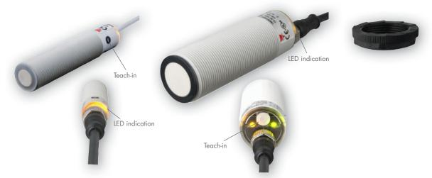
UA18: M18 x 83.6 mm (Cable) UA18: M18 x 77.7 mm (Plug) UA30: M30 x 89.5 mm (Cable) UA30: M30 x 89.5 mm (Plug) All UA30 models include a locknut with retention grips for tight mounting.
