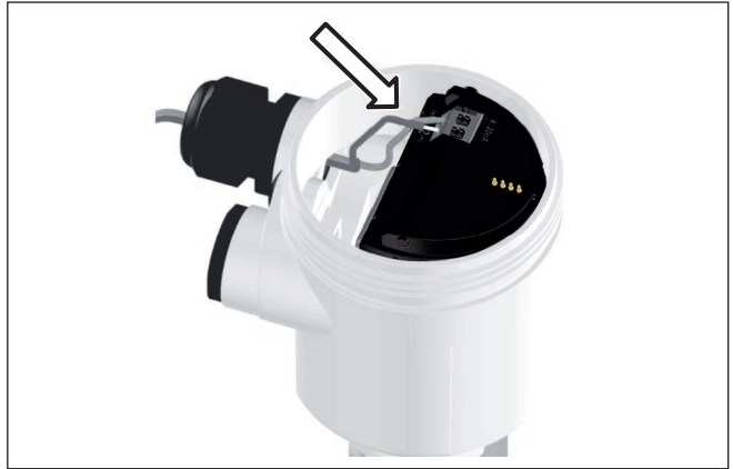
Fig. 18: Connection steps 5 and 6 - Single chamber housing
