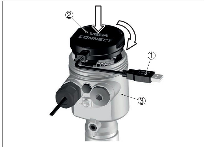
Fig. 31: Connection of the PC directly to the sensor via the interface adapter
