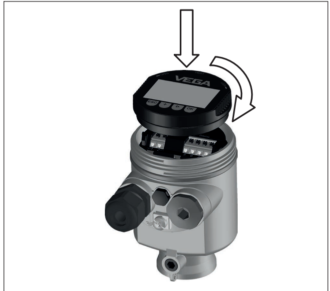
Fig. 14: Installing the display and adjustment module in the electronics compartment of the single chamber housing
