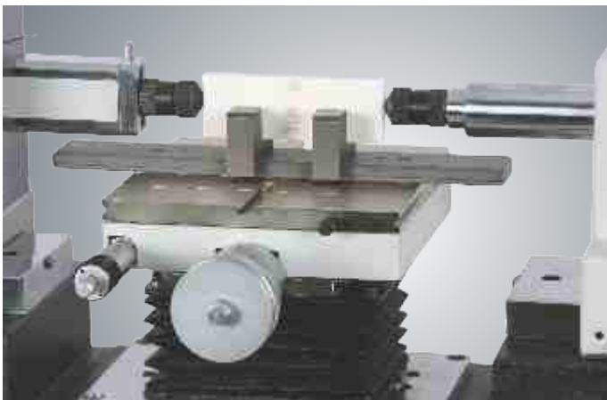
Gauge block measurement : Hold on table by using holding attachment
