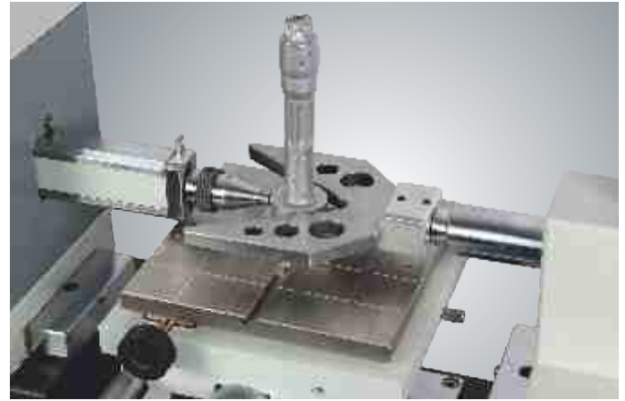
Internal micrometer (3 point) Calibration : By using V reference standards and Flat anvil.
