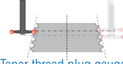
Taper thread plug gauge measurement of d2 by using single arm measurement attachment
