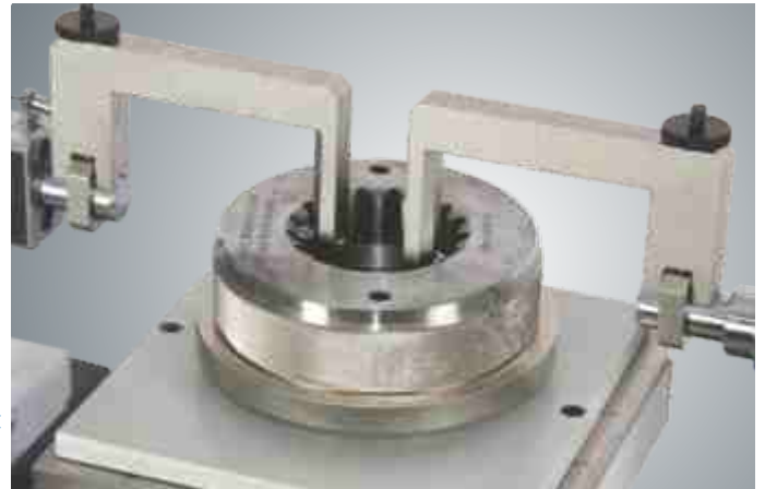
Spline ring gauge measurement by using fixed dual arm and precision spherical styli : Hold on floating table.
