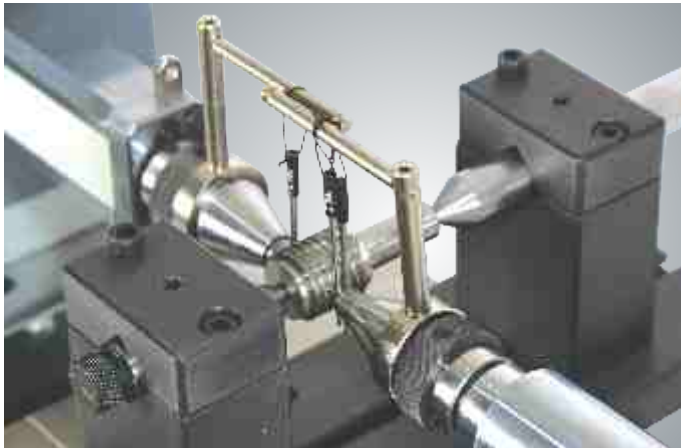
Cy. Thread Plug Gauge (below 100 mm) measurement : Hold between center table
