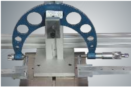
External Micrometer (above 150 mm) Calibration : Hold on universal holder.
