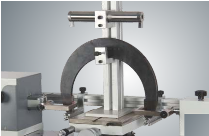
Snap Gauge C Type (above 300 mm) measurement : Hold on universal holder
