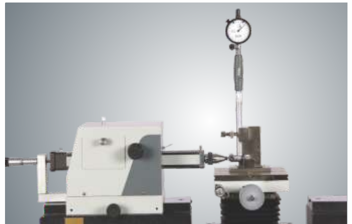
Bore Gauge Calibration : Hold on table by using holding attachment and machine spindle drive unit.
