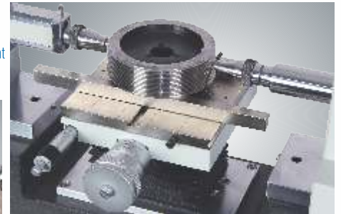
Cy. Thread Plug Gauge Measurement of Effective diameter Below 40 mm : Hold in Vee block holder
