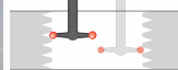
Thread ring gauge measurement of Effective Diameter (D2) by using single arm measurement attachment with single axis bi-directional probe & T-shape stylus
