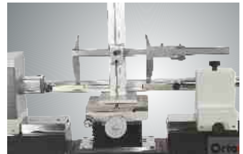
Caliper Calibration : Hold on universal holder
