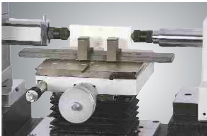
Spline plug gauge measurement by using cylindrical pins and a pair of flat anvils
