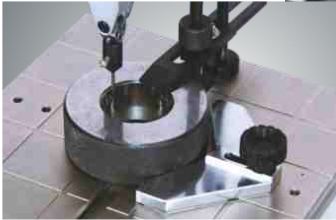
Plain ring diameter (above 2 mm) measurement : Using a Single Ruby Ball Stylus with bi-directional probing system of single arm measuring attachment
