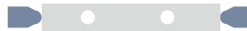
Gauge block / Length Bar measurement by using a pair of ball anvils
