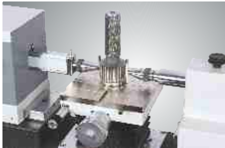
Spline plug gauge measurement by using cylindrical pins and a pair of flat anvils
