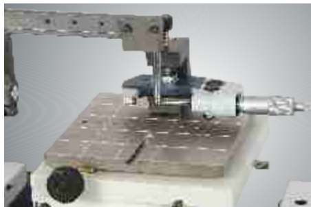
External Micrometer (Below 150 mm) Calibration : Hold on table by using C clamp
