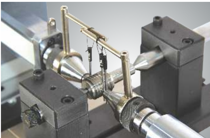
Cy. Thread Plug Gauge measurement : Hold between center table
