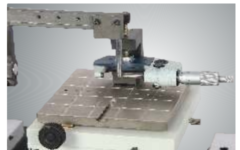
External Micrometer (Below 150 mm) Calibration : Hold on table by using C clamp and measurement by using universal measuring arm
