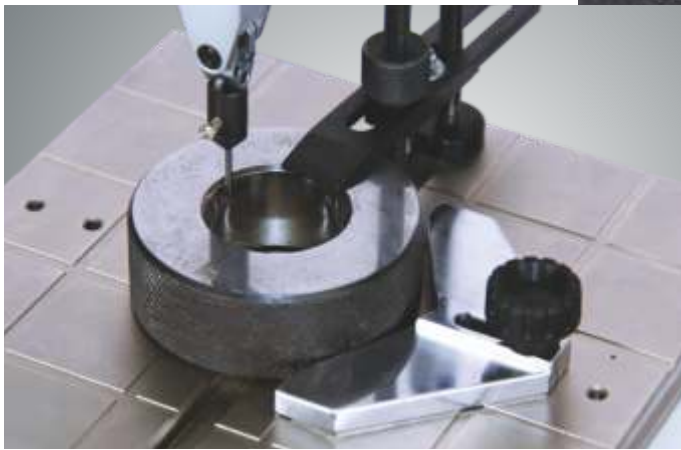
Plain ring diameter (above 1 mm) measurement : Using electric measuring arm.
