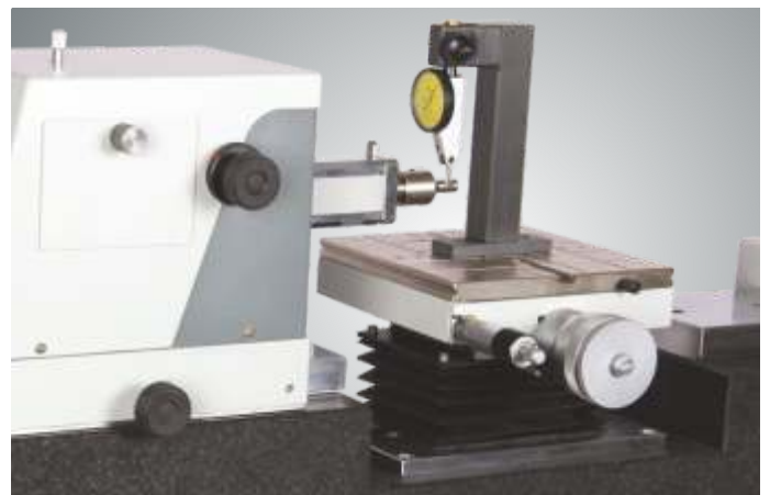
Dial Test Indicator Calibration : Hold on table by using holding attachment
