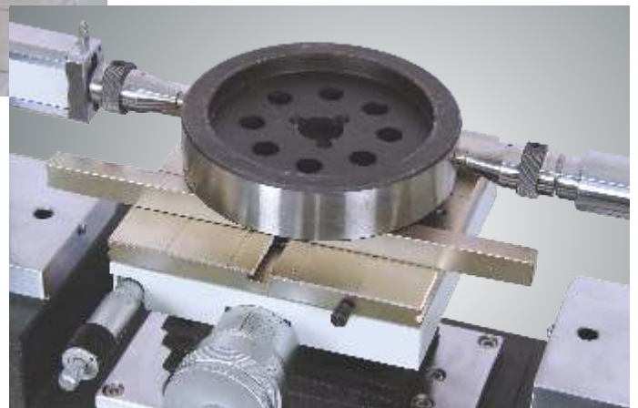
Plug Gauge (above 40 mm) measurement : Hold on parallel blocks
