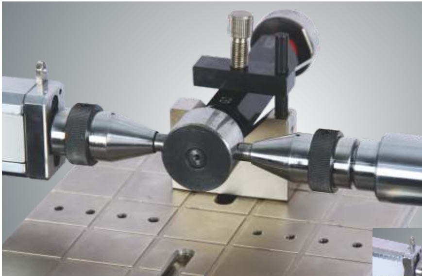
Plug Gauge (below 40 mm) measurement : Hold in Vee block holder
