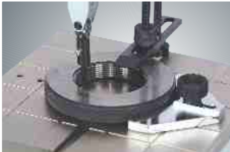
Cy. Measurement of effective diameter by using single arm measuring attachment & Precision Ruby T-Shape styli
