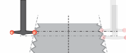
Taper thread plug gauge measurement of d2 by using single arm measurement attachment
