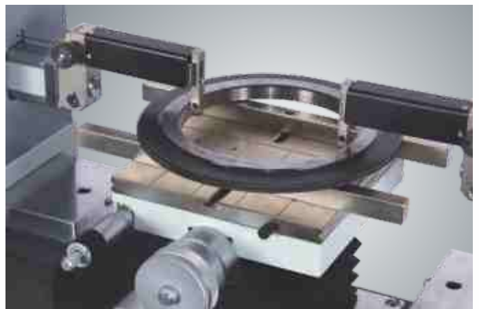
Cy. Thread Ring gauge measurement of effective diameter by Precision Ruby ball styli and flexible dual measuring arms
