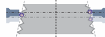
Taper Thread plug gauge measurement of d2 by using thread measuring wires and a pair of flat anvils
