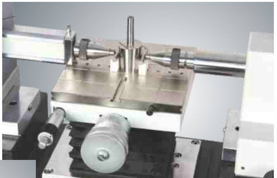
Taper plug gauge measurement : By using cylindrical pin gauges (over pin measurement)
