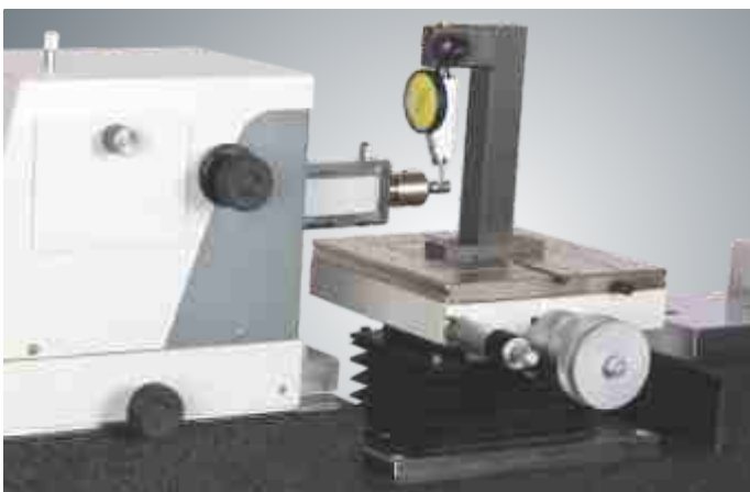
Dial Test Indicator Calibration : Hold on table by using holding attachment
