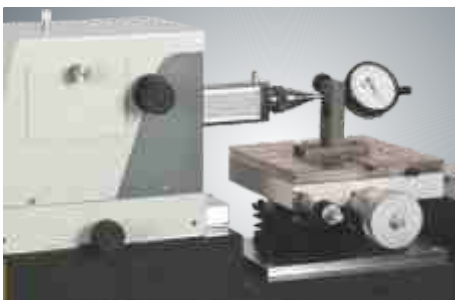
Dial Indicator Calibration : Hold on table by using holding attachment
