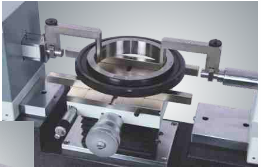
Plain ring diameter (above 10 mm) measurement : Using a pair of fixed arms
