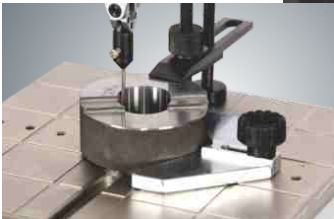
Taper ring gauge measurement : Using a Single Ruby Ball Stylus with bi-directional probing system of single arm measuring attachment
