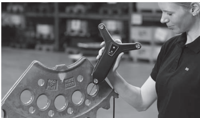
The hand-held ZEISS T-POINT touch probe – the ideal portable coordinate measuring machine for simple single-point measurements
