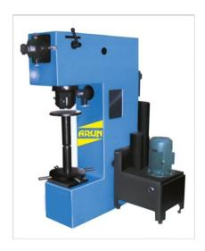
Basic machine design & operation similar to B-3000 (H). In addition 'optical device' with 14 x magnification provided in front to project dia of ball impression on glass screen with a micrometer measuring system with 0.01mm accuracy. The indentor swivels & projects dia of ball impression immediately after unloading operation which avoids additional time for measurement of ball impression
