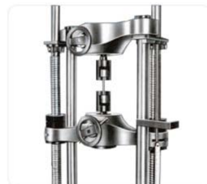
Attachment for Tension Test for shouldered and threaded specimens
