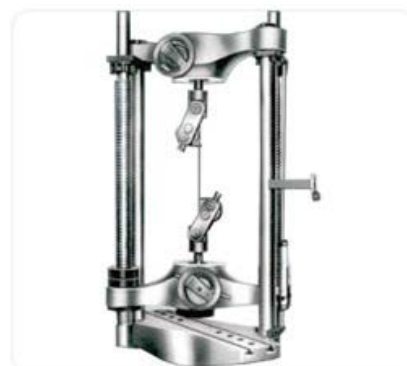
Attachment for Tension Test for Wire Ropes
