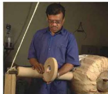
Taping of PT Coil
