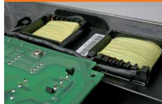
DC coils reduce harmonic noise and protect the drive
