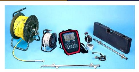
Monitoring of lateral earth movements in landslide areas
