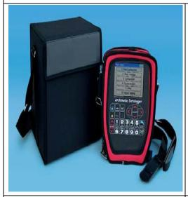
Archimede is a battery operated datalogger with a large graphic color backlight display, housed in a crushproof, water-resistant plastic case. This datalogger has been specially designed for field use in heavy operating conditions. A convenient remote handswitch allows one-man surveys. Its powerful display is able to show a preliminary inclinometer graphs on field.
