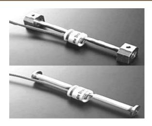
Systel Series 1000 model Strain Gage is designed to measure the changes in strain in and on structural members associated with many types of structure. Concrete Dams Buildings over tunnelling works Deep Excavations Retaining Walls Bridges Pile caps Suitable for portable readout equipment or automatic data acquisition.
