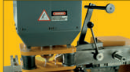
Optional 'drive-in' minimum deform stripper and bolster assemblies.
