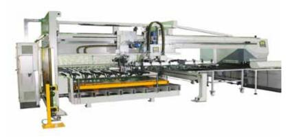
The 3015 SHEET TRANSFER System is designed for loading of sheets from a pallet onto the CNC Punching Machine, and the unloading of the punched sheet from the machine table onto a stacking unit.
