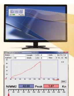
Two way communication to machine i.e. machine can be start, stop and controlled from the computer
