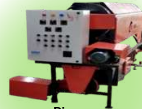
Biomass Torrefaction Plant (Charcoal Plant)
