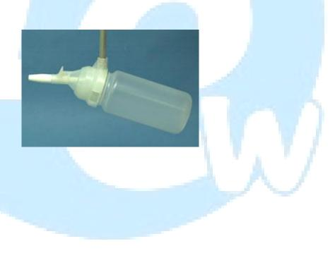
The US DH-5912 is a medium-weight hand-line suspended-sediment sampler. The sampler can be lowered and raised, hand over hand, with a flexible suspension line. It can be used in stream depths up to 15 ft and in steam velocities ranging from 1.5 to 5.0 ft/sec.
