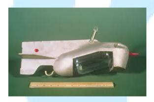
The US DH-76 is a medium-weight hand-line suspended-sediment sampler. The sampler can be lowered and raised, hand over hand, with a flexible suspension line. It can be used in streams with depths up to 15 ft and in stream velocities ranging from 1.5 to 6.6 ft/sec. The US DH-76 is similar in design to the US DH-59, but uses a quart glass bottle for additional sample volume, as opposed to the pint bottle used in the US DH-59.
