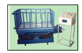
Note: vibration tester as per IS 7028 for bottle of 20 Ltr. Capacity. We will Provide vibration meter in panel. Range 0.6Hz. and 1 Timmer for Time setting
