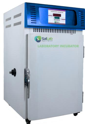
SaiLab Equipment's **Laboratory Incubator** provides a temperature - controlled environment for the growth of microbes. The incubator has a double-walled construction with an outer body that is MS powder - coated. It comes with a PID controller for accurate temperature control and a safety thermostat. The equipment is secured with glass wool insulation and has an audible alarm.
