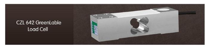
Model CZL 642 (Platform ( $25mm \times 25 mm$ ) - Greenlable) is strain gauge based loadCell constructed from Aluminum Alloy. It is economical and low profile cell. It is mainly used in check weighing. Suitable for Platform size upto 500mm X 500mm.
