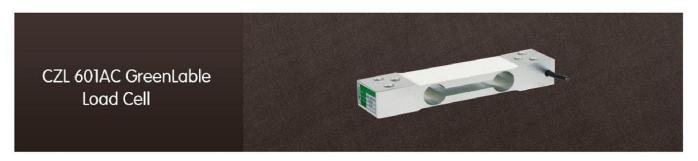
Model CZL 601AC (Table Top- Greenlable) is strain gauge based LoadCell constructed from Aluminum Alloy for high Accuracy. It is mainly used in check weighing. Suitable for Platter size upto 400mm X 400mm.
