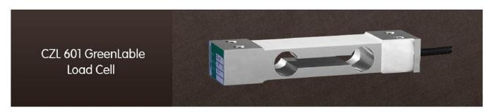
Model CZL 601 (Table Top- Greenlable) is strain gauge based LoadCell constructed from Aluminum Alloy for high Accuracy. It is mainly used in check weighing. Suitable for Pan size upto 250mm X 350mm.
