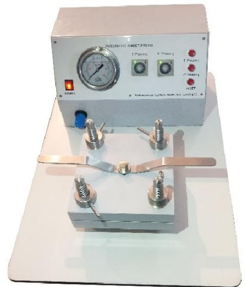
Usage : Pressing and Dewatering sheet made on sheet making machine.
