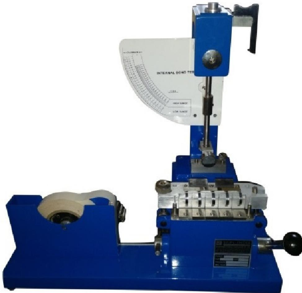
Usage : Determines the internal bonding of paper and board .
