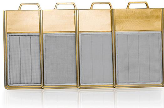
Usage: for determining the fibre length of pulp by classification.
