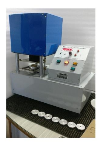
Usage: for measuring the compressive strength of board and corrugated board.
