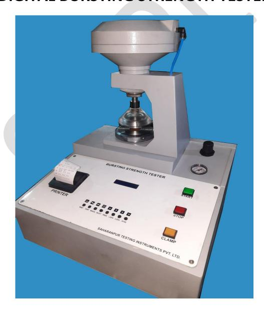
Usage: for determining bursting strength of paper and board
