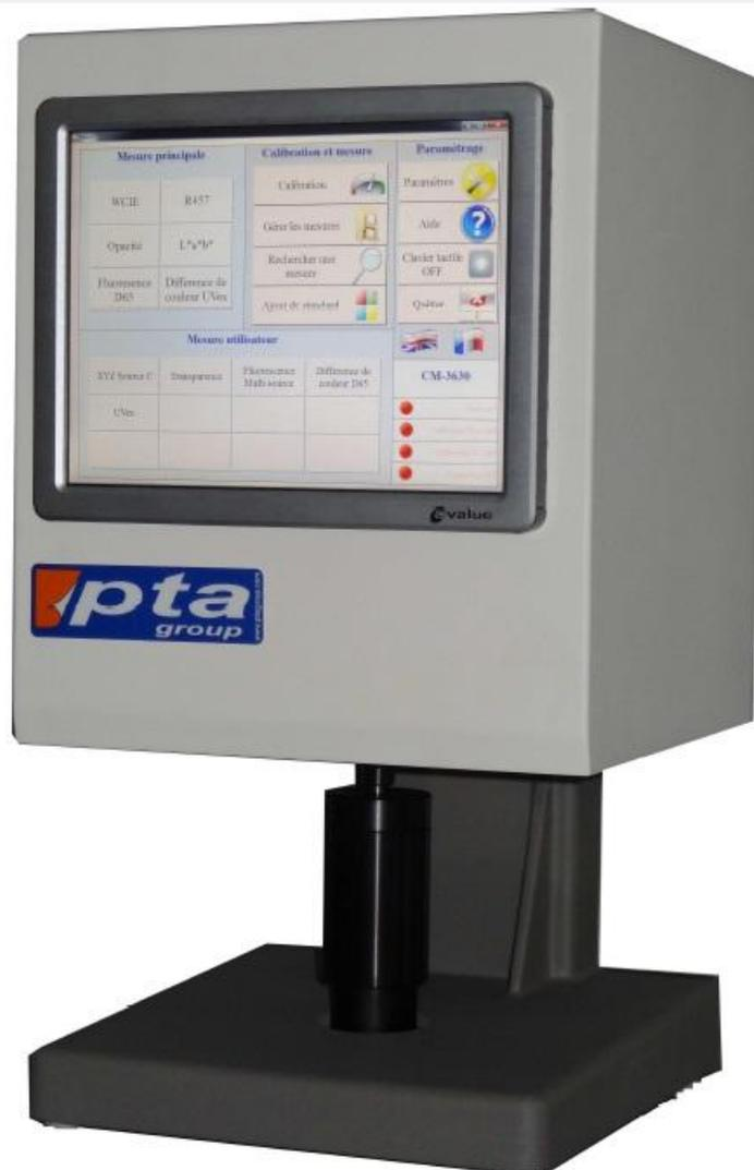
Usage : for measuring the ISO Brightness , colour , colour difference , fluorescence and opacity of paper.
