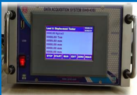
Data Acquisition System with Pile Load
