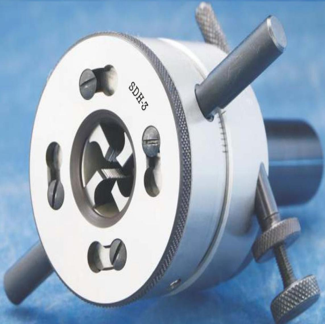
Mounted on center lathes, capstans, turrets or like machine tools 'TACO' self opening die-heads are used for cutting threads and are most suitable for heavy duty work & mass production. Die-heads open automatically when the selected thread length is reached eliminating the necessity of the direction or working spindle.
