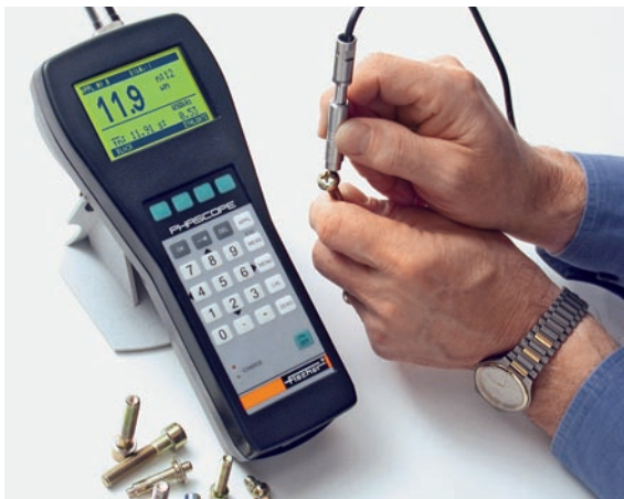
The ESD2.4 probe is particularly well-suited for small parts, because re-calibration for the specific measuring spot geometry is typically not required
