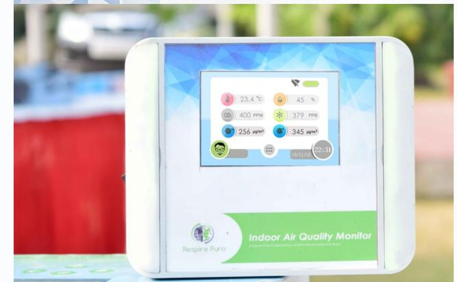
The RP-IAQ Indoor Air Quality Monitor features a simple-to-use, HMI touchscreen display along with Hexa-monitoring of indoor air quality parameters (PM2.5, PM10, carbon dioxide, volatile organic compounds, along with temperature and humidity). The monitor has been designed respective to ease of installation and handy in use/porting.
