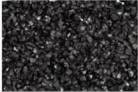
Activated carbon is a granular material produced mostly by roasting charcoal from coconut shells or coal at 800 to 1000°C to "activate" it. Impurities are removed by acid washing. Typically, it has pore sizes ranging from 500 to 1000nm and a surface area of about 1000m2/gram. A much purer form of activated carbon is produced by paralyzing polymer beads.
