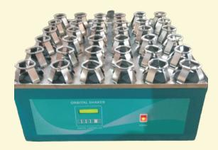
Body is made of Heavy M.S. powder coated with Stainless Steel tray for flask.
