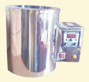
Double walled construction. Inside made up of stainless steel.
