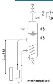
Operating and installation diagram for a SBF6000 system.
