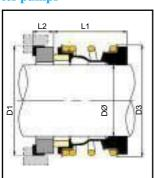
MAK-TECH SEALS manufacture and stock a range of elastomer bellow seals to suit the common Types of K.S.B.® "ETA-" series centrifugal pumps commonly found thoughtout the fluid industry.
