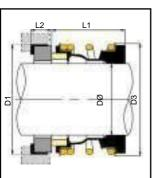
MAK-TECH SEALS manufacture and stock a range of elastomer bellow seals to suit the specific dimensions of K.S.B.® "AMA-", "KRT-" and "SEWA-" series waste-water pumps with "SU-" prefix seals installed. 25mm size is commonly used in the 'oil bath' position, with 22mm MTS EBG1 in the 'outer' position, 33mm sizes are used in pairs in the same pump series. 28mm is commonly used in "Vitachrom" pumps in tandem with MTS 127B.
